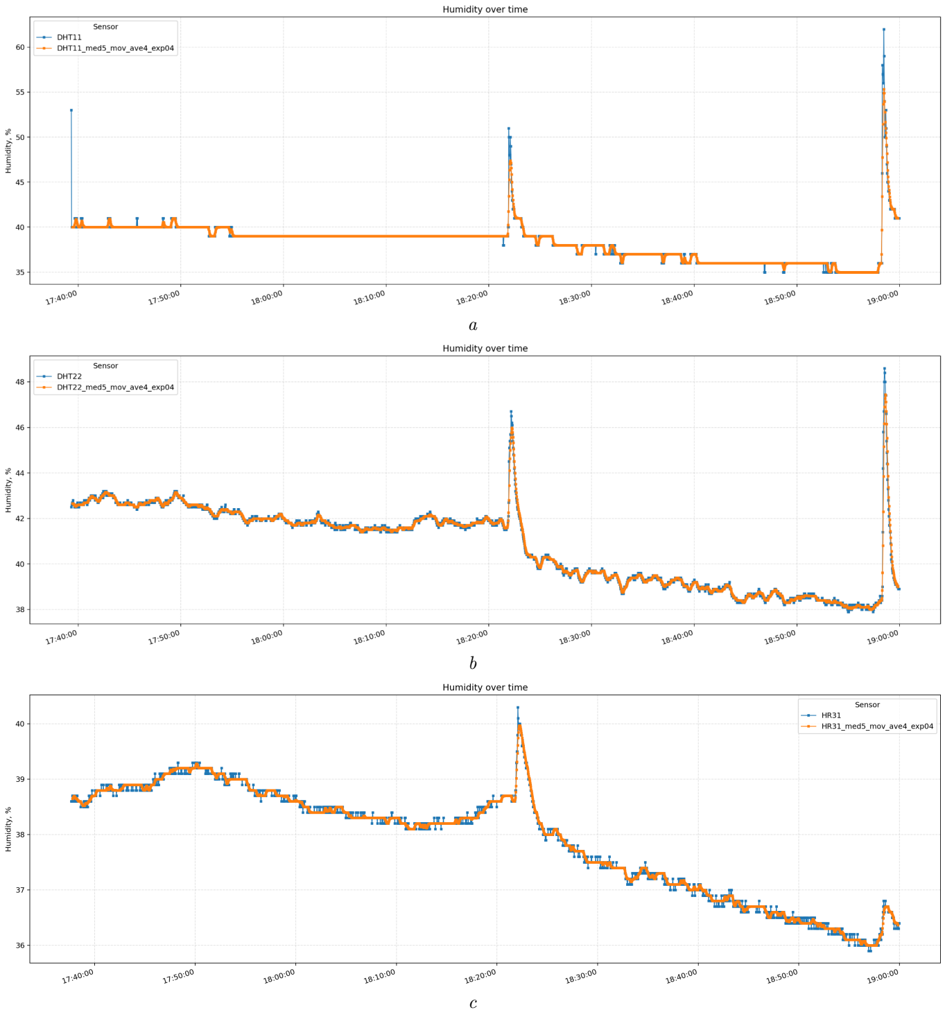
Fig. 5. Comparison of humidity before and after treatment: a – DHT11 sensor; b – DHT22 sensor; c – HR31 sensor
