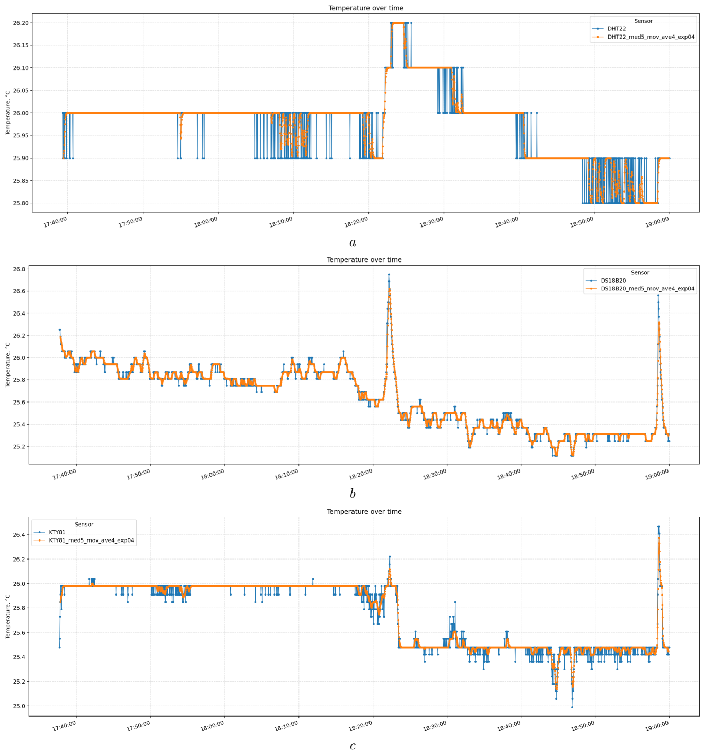
Fig. 8. Comparison of temperature from multiple sensors before and after processing: a – DHT22 sensor; b – DS18B20 sensor; c – KTY81 sensor
