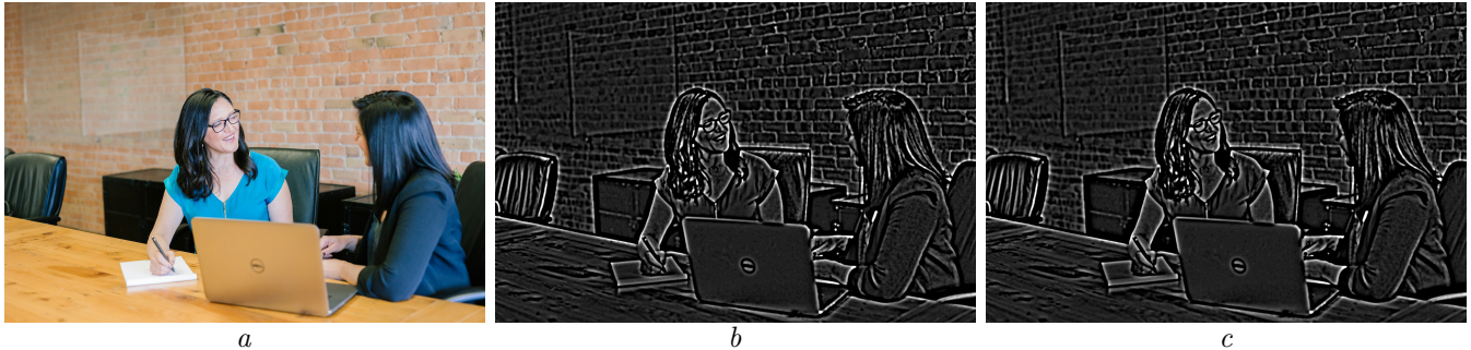
Fig. 2. Qualitative comparison of full DoG outputs: a – Input image; b – DoG (FIR); c – DoG (IIR)
